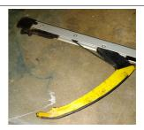
The only problem that tends to happen is that the knot slips or the cord stretches, meaning that the jaw will not close properly. Sometimes the cord slips off one or both of the pulley wheels as a result.
