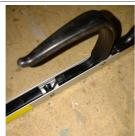
At the handle end the cord passes through a hole in the trigger either with a metal piece crimped onto it or a knot to stop it coming out.
